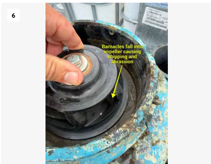
Barnacles fall into impellor causing the chips in the impellor.
