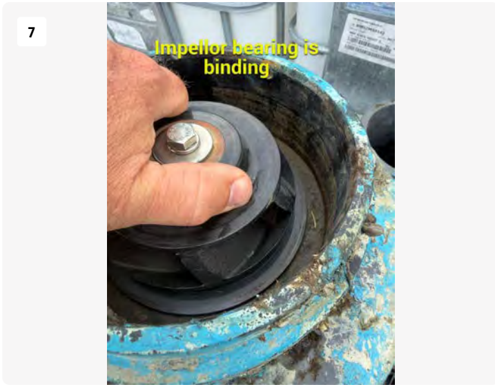
Impellor bearing is binding.
